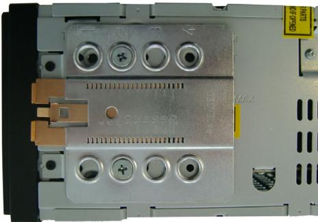
The bracket mounted on the car radio.
