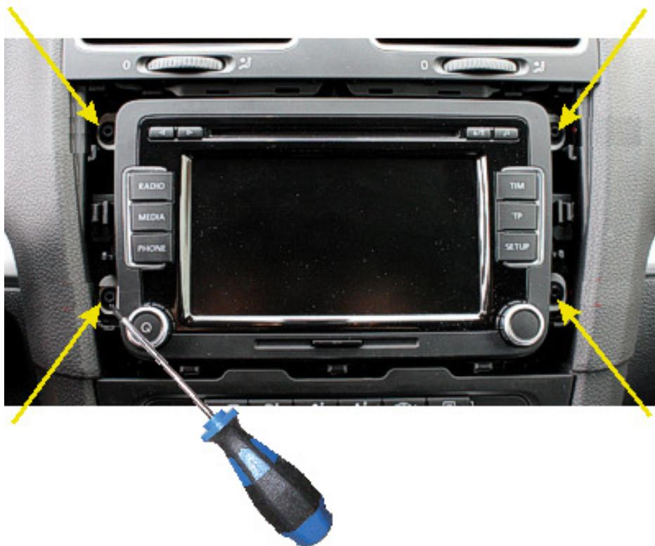
2. Use a screwdriver to undo the four indicated Torx screws (T20).
