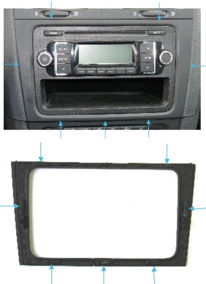
The disassembled panel has retaining lugs on the rear.
