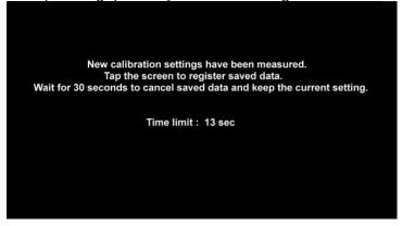
Tap on the screen within 30 seconds to save the calibration to the device, to save the data.
